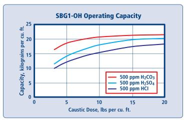
Capacity based on 500 ppm of stated acid (as CaCO<sub>3</sub>). Capacity based on 36 inch deep bed depth, flow rate of 2 to 4 gpm per cu. ft. and greater than 40 minute caustic injection time. No engineering downgrade has been applied.
